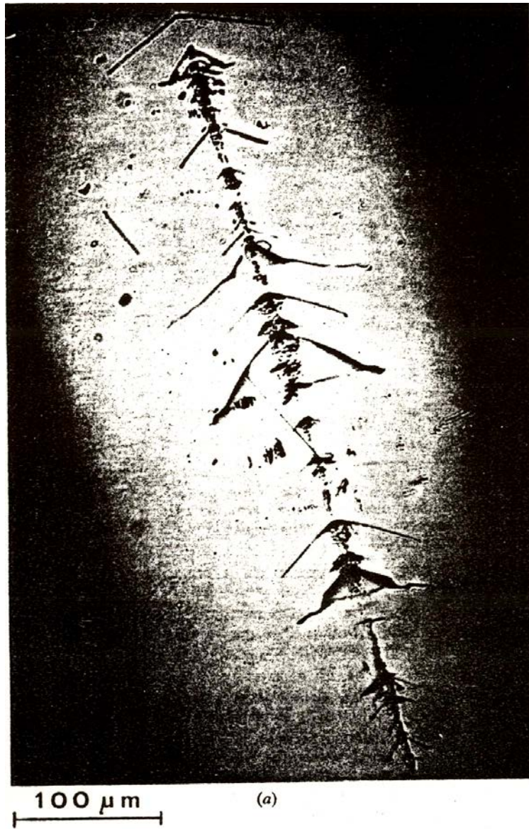
Figure 6.7. (a) Surface damage produced by light abrasion of one glass rod on another
