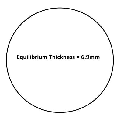
When molten glass is poured onto tin, it will spread until the interfacial tensions and gravitational forces are balanced, resulting in a circular glass-tin interfacial shape with an equilibrium thickness of 6.9mm.
