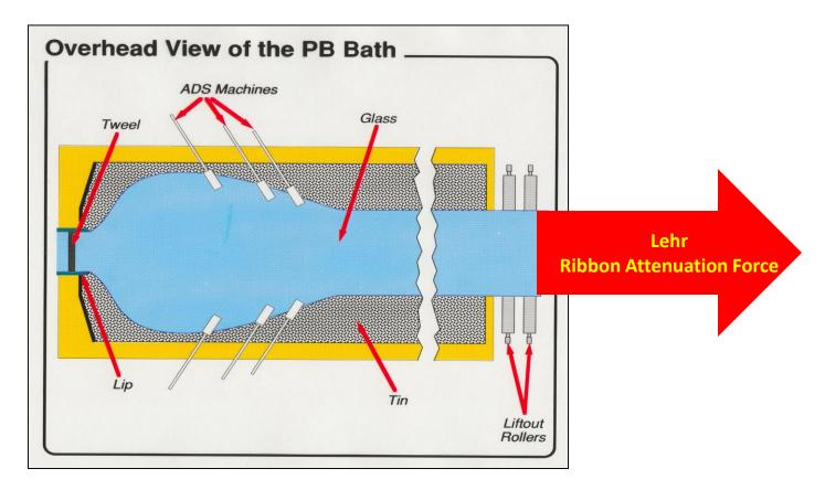
Glass flows onto the tin at a thickness of approximately 5 cm and spreads to achieve an equilibrium thickness of .6858 cm.
