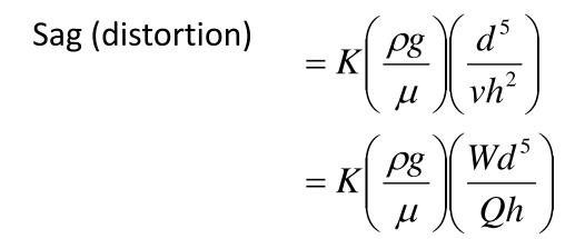
Thus, exit end distortion is inversely proportional to the ribbon viscosity and the ribbon thickness.
