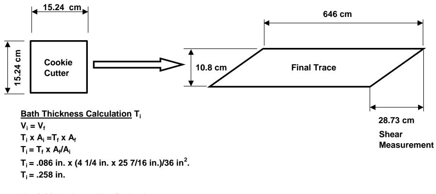
$V_i$  = initial volume  $V_f$  = final volume  $T_i$  = initial thickness  $T_f$  = final thickness
