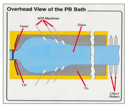
Glass flows onto the tin at a thickness of approximately 5 cm and spreads to achieve an equilibrium thickness of .6909 cm.
