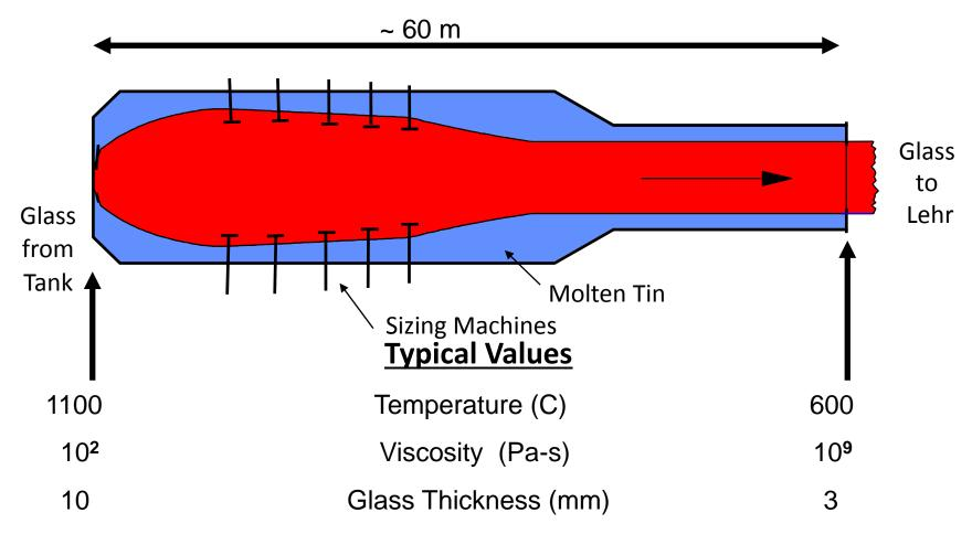
Massive glass viscosity variation 1:10<sup>7</sup> Glass aspect ratios are large - Length:Width:Thickness = 10,000:1,000:1
