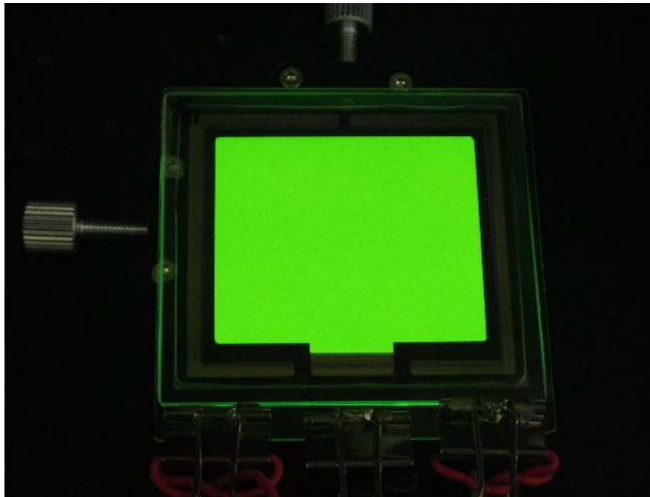
Device structure Glass /IZO,100/ND1501,40/NPD,50/Ir(ppy)<sub>3</sub>+CBP[6%],30/BAIq,10/Alq,30/LiF,0.8/Al,150
