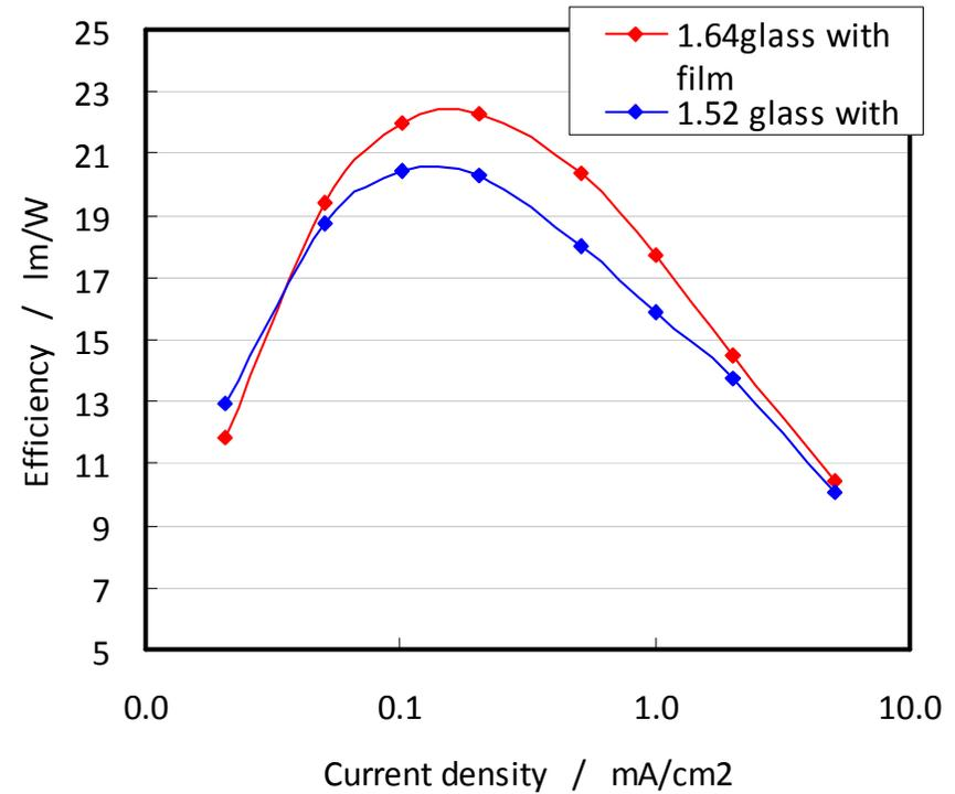
Device structure Glass / IZO,100/ND1501,40/NPD,50/Ir(ppy)<sub>3</sub>+CBP[6%],30/BAIq,10/Alq,30/LiF,0.8/Al,150
