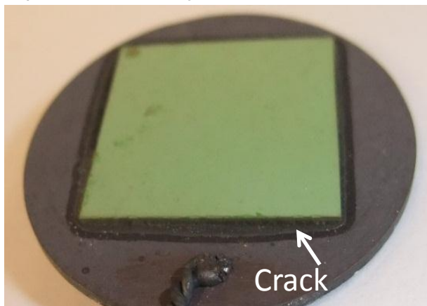
Cracked on quenching (>25° C/s)
