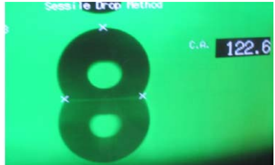
Photograph of water bead on the C-assisting sputtered TiO 2 film
