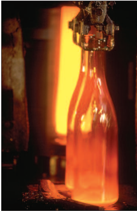
FIGURE 3 A silicate melt emerging from an industrial furnace and being transformed into a bottle. PHOTO COURTESY OF SAINT-GOBAIN COMPANY
