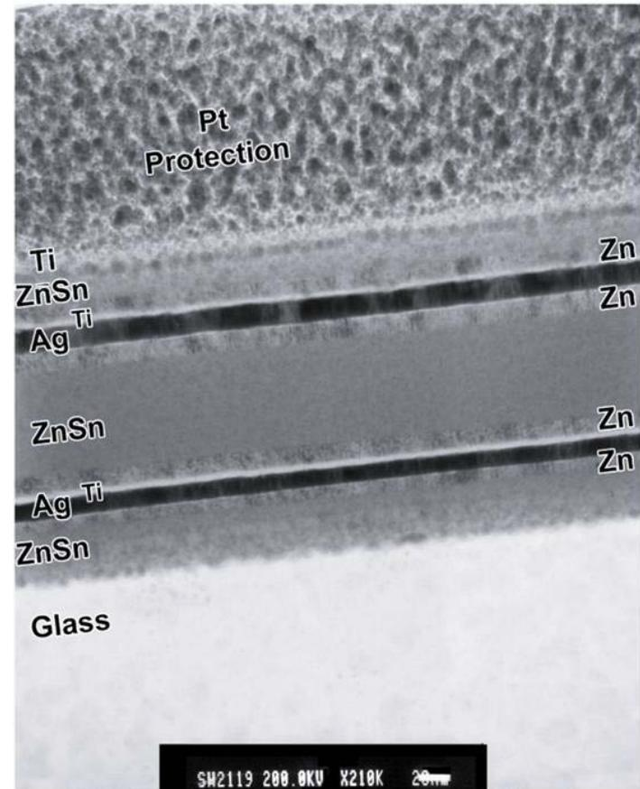
Figure 3 XTEM image of a good area of sample 103285 showing full film stack.
