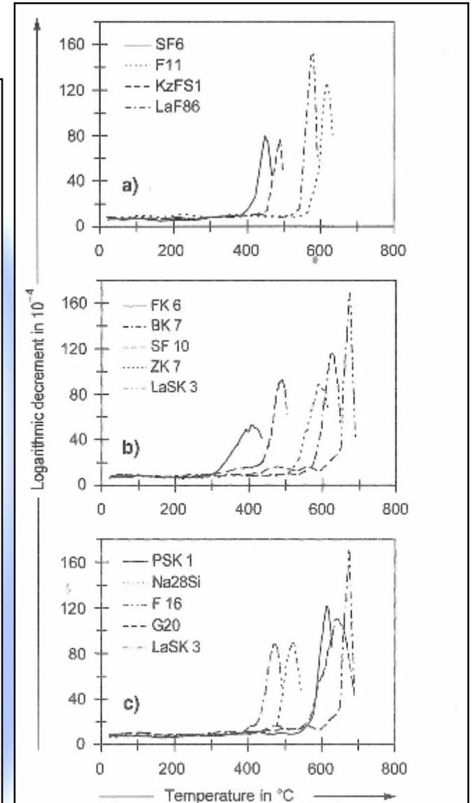
Figures 4a to c. Logarithmic decrements of the coupled system pendulum-specimen bar for different glasses ( $f_p = 0.79$  Hz), a) SF6, LaF86, KzFS1 and F11; b) FK6, BK7, SF10, ZK7 and LaSK3; c) PSK1, Na28Si, F16, G20 and LaSK3.
