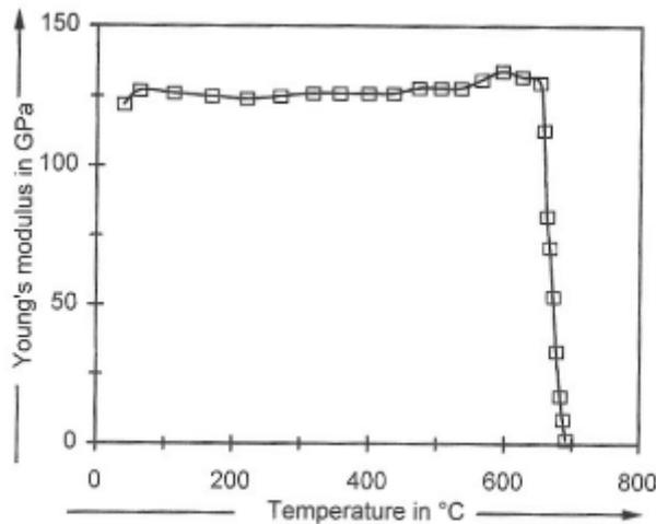
Figure 5. Young's modulus of the glass LaSK3 in dependence on temperature.
