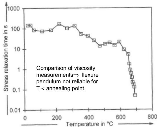
Figure 6. Stress relaxation time of the glass LaSK3 in dependence on temperature.
