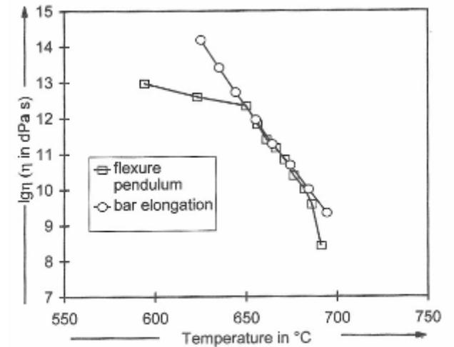
Figure 9. Comparison of the viscosities obtained by means of the flexure pendulum equipment and with the help of the bar elongation method, in dependence on temperature, example glass LaSK3.
