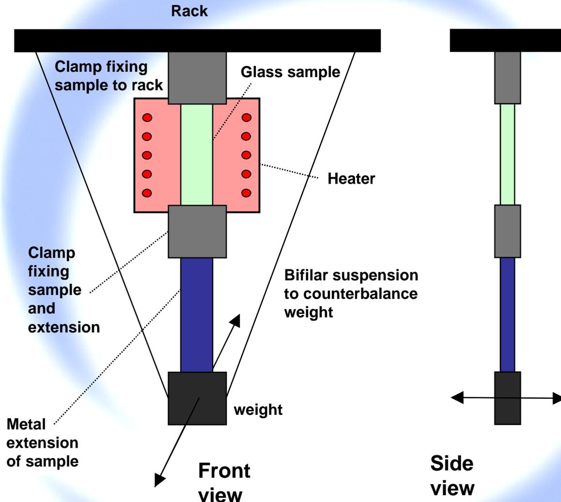
The flexure pendulum monitors self oscillations in a bending mode.
