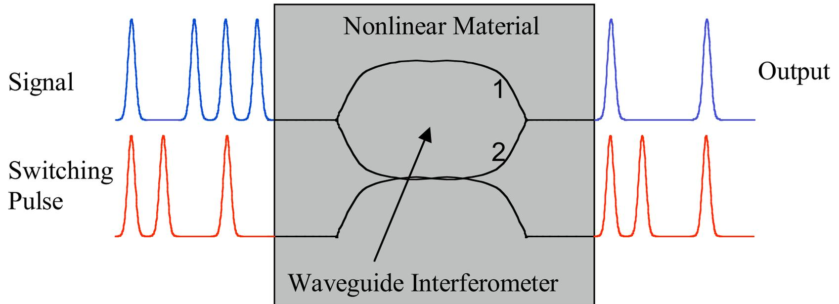
Without switching pulse: waves in leg 1 and 2 interfere destructively, no output
