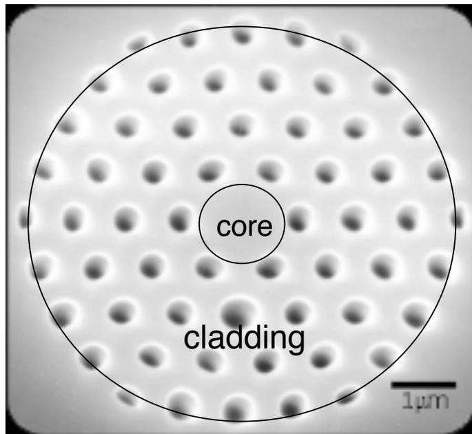
propagation of pulsed (100fs) Ti-sapphire laser light( 800 nm) results in supercontinuum generation : 400-1600 nm
