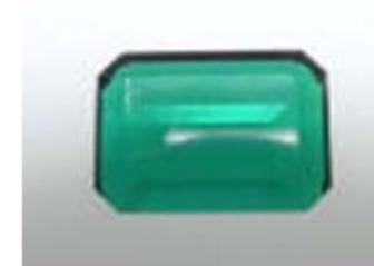
Beryl ( $\text{Be}_3\text{Al}_2\text{Si}_6\text{O}_{18}$ ) with 1% of Cr impurity substituting Al in octahedral sites.
