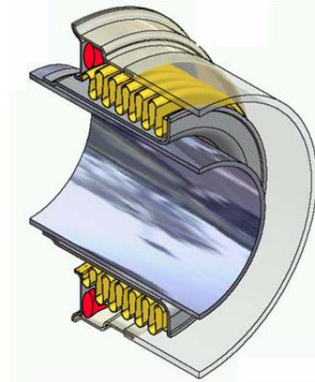
The **third issue** is the improvement of the **borosilicate glass** receiver resistance to **acid rain**. In fact, the **degradation of functional materials** and consequent loss of performance is a **crucial factor** for the economic viability of **solar systems**, which are severely **exposed to the unpredictable outdoor weather**.
