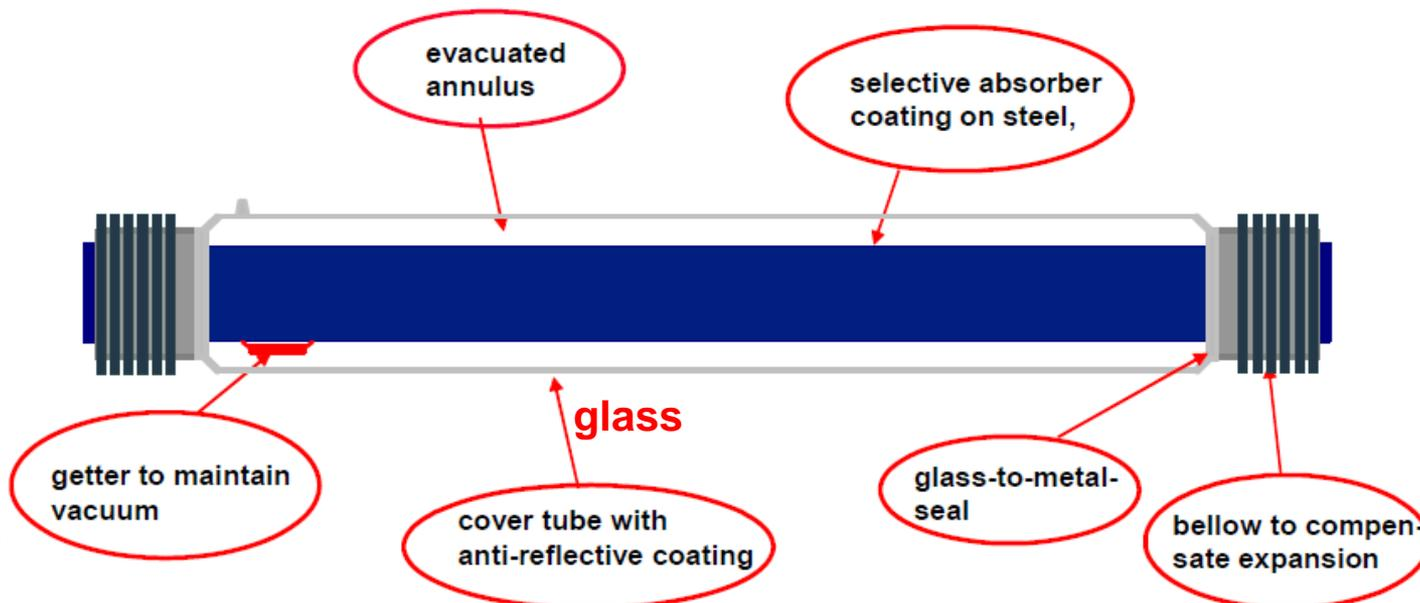
The **metal receiver** should be designed **to minimize heat loss**. Heat retention by the receiver is enhanced by covering the metal receiver with a selective (**low-E**) coating which will absorb virtually all the concentrated radiation, but will reradiate little energy back.
