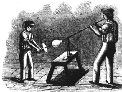
Figure 2. The glass blower enlarging the glass flask, assisted by his helper in keeping the mass of molten glass centered. (From ref 7.)
