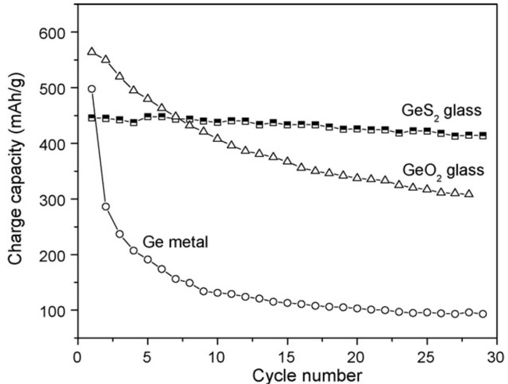
Fig. 5. Cycle-life performance of Ge metal, GeO<sub>2</sub> glass, and GeS<sub>2</sub> glass, respectively. They are operated between 1.5 and 0 V at the rate of 0.1 C.
