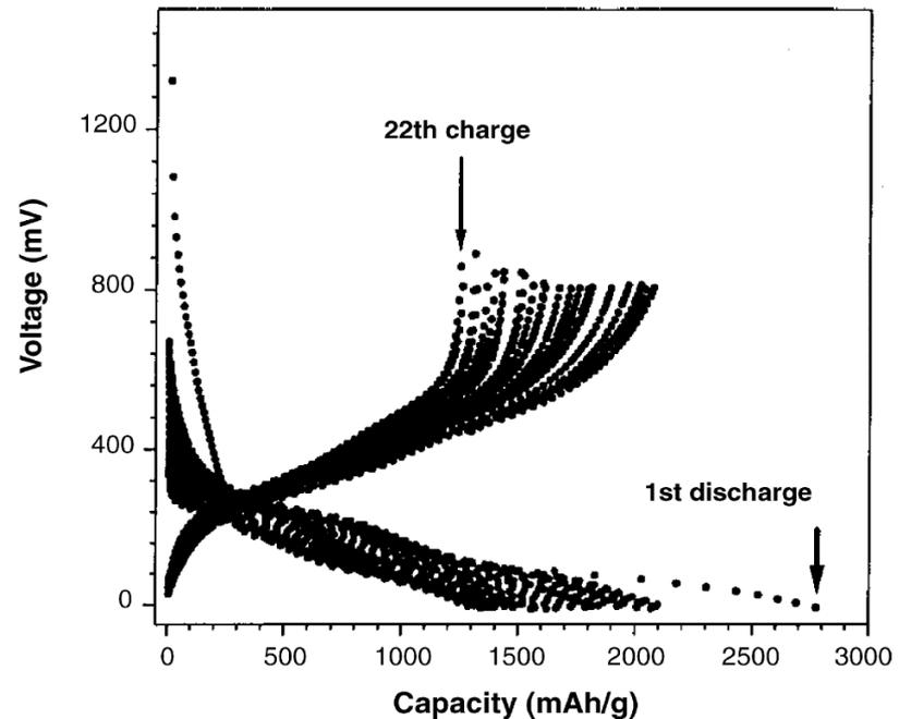
Fig. 5.  $\text{§§}$  Charge-discharge curves between 0.0 and 0.8 V at  $0.1 \text{ mA cm}^{-2}$  for nano-Si anode with 4:4:2 weight ratio of nano-Si, carbon black and PVDF binder. Electrolyte: 1 M  $\text{LiPF}_6$  in ethylene carbonate (EC)-diethyl carbonate (DEC) (1:1) [22].
