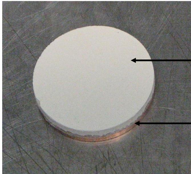
Targets are attached onto a copper plate by silver paste
