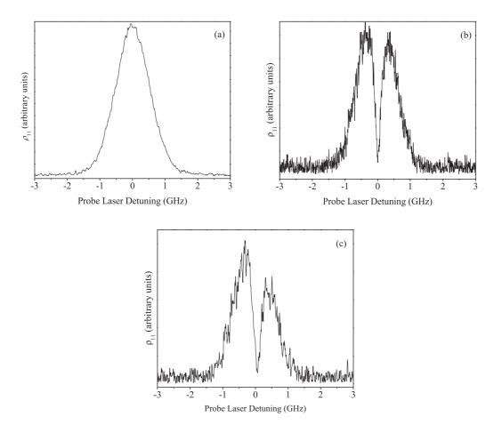
FIG. 3. Experimental spectra for  $Na_2$  V-system probe laser scans in the copropagating geometry (a) with the coupling field turned off and (b) with the coupling field on and the frequency of the coupling laser set to line center of the transition. (c) The coupling field is detuned by  $\sim$ 60 MHz. The coupling laser power is 265–270 mW and the probe laser power is less than 1 mW.
