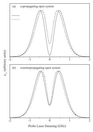
FIG. 10. Comparison between (a) co- and (b) counterpropagating fluorescence signals for the cases of  $\rho_{13} \neq 0$  (solid line) and  $\rho_{13} = 0$  (dashed line) in an open 3-level V-type system. The calculation of the population of level  $|1\rangle$  is carried out using parameters close to the experimental conditions:  $\Omega_1/(2\pi) = 10$  MHz,  $\Omega_2/(2\pi) = 220$  MHz,  $\gamma_{ij}^{col}/(2\pi) = 0.79$  MHz.
