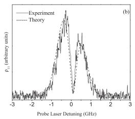
FIG. 8. Experimental (solid line) and simulated (dashed line) data for copropagating beams. By inserting the real experimental parameters in our density matrix equations we simulate the experimental data when (a) the coupling field is on resonance with  $\Omega_2/(2\pi)=220$  MHz and (b) the coupling field is detuned 100 MHz with  $\Omega_2/(2\pi)=190$  MHz. The probe laser Rabi frequency  $\Omega_1/(2\pi)$  was 10 MHz in both cases.
