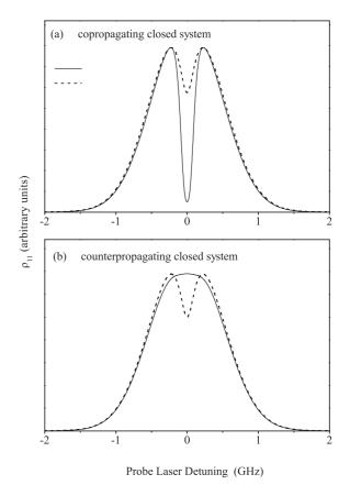
FIG. 11. Comparison between (a) co- and (b) counterpropagating fluorescence signals for the cases of  $\rho_{13} \neq 0$  (solid line) and  $\rho_{13} = 0$  (dashed line) in a closed 3-level V-type system. The calculation of the population of level  $|1\rangle$  is carried out using parameters close to the experimental conditions:  $\Omega_1/(2\pi) = 10$  MHz,  $\Omega_2/(2\pi) = 220$  MHz,  $\gamma_{ij}^{col}/(2\pi) = 0.79$  MHz.
