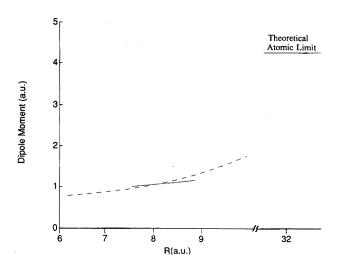
FIG. 11. Comparison of the relative dipole moment obtained in the present work (solid line) with the theoretical dipole of Ratcliff *et al.* (Ref. 27) (dashed line). The experimental D(R) was normalized to the Ratcliff *et al.* result at R = 8.034 a.u. The flat line of the theoretical curve to the right represents the asymptotic theoretical dipole moment.
