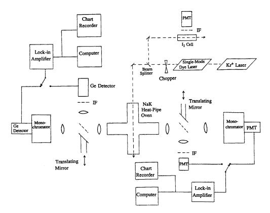
FIG. 5. Experimental setup. IF and PMT represent interference filter and photomultiplier, respectively.
