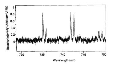
FIG. 7. *P-R* doublets of the downward  $2^{1}\Sigma^{+}$  (v' = 20, J' = 37)  $\rightarrow 1^{1}\Sigma^{+}$  (v'', J'' = 36,38) transitions. The upper state was pumped from the v'' = 0, J'' = 36 level of the  $1^{1}\Sigma^{+}$  state. Typically these *P-R* doublets extend to approximately 1.0  $\mu$ m.
