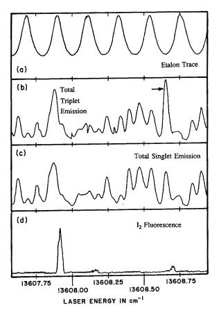
FIG. 6. Excitation spectra. (a) laser etalon signal indicating the continuity of the scan. (b) total triplet band emission. (c) total singlet emission. (d)  $I_2$  fluorescence. The arrow in (b) indicates a position of enhanced triplet emission and therefore a perturbed energy level.
