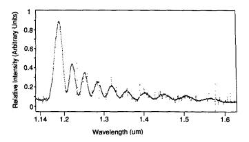
FIG. 8. Bound-free emission from the  $1{}^{3}\Pi_{1}(v'=18, J'=37)$  level. This spectrum was obtained with the same pump wavelength used to produce Fig. 7.
