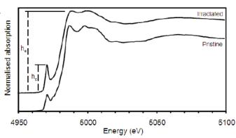
From the increase in the 3d peak just above 4970 eV and the damping of higher energy oscillations, we obtain quantitative data on these local structural changes.
