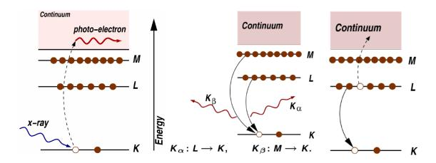
The figure on the left shows a schematic of the photo-absorption process. The core-hole is eventually refilled by a higher-lying electron, resulting in the emission of a secondary photon (middle) or of an Auger electron (right).
