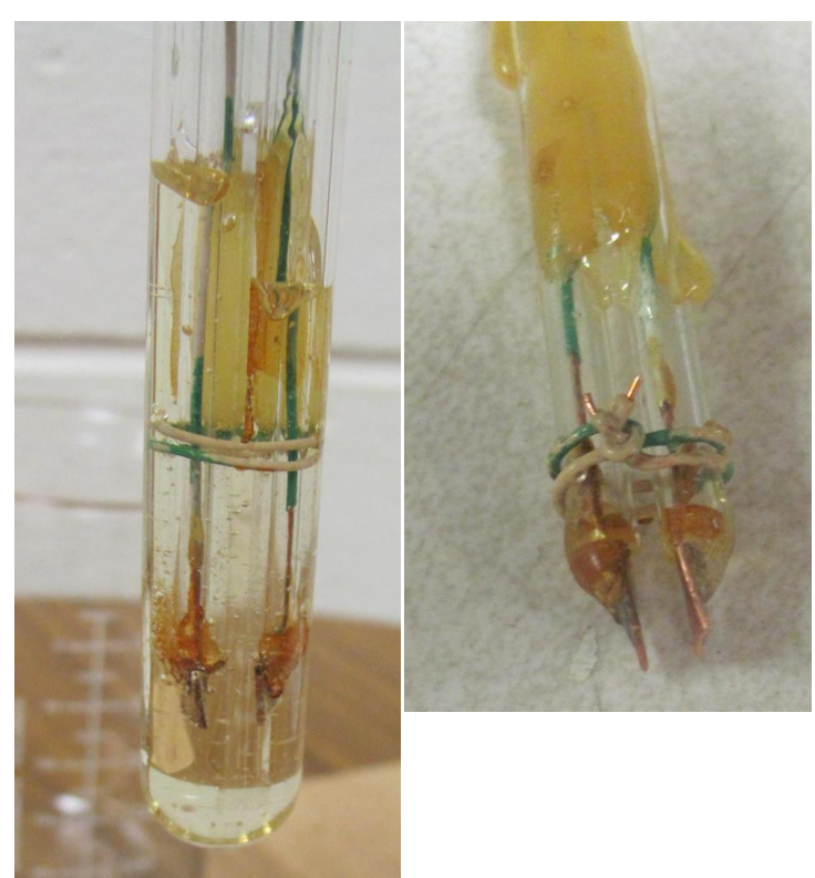
Cell Constant (Area/spacing) = 0.715 cm
