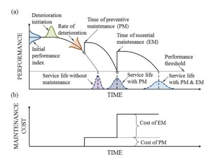
$Deterioration\ and\ maintenance\ effects\ on\ performance\ and\ cost$
