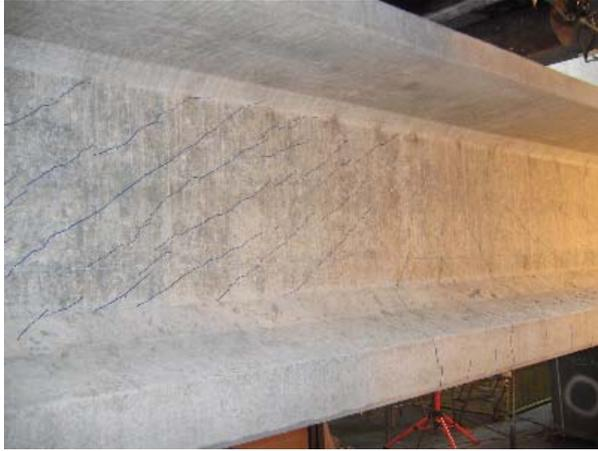
c) Shear cracking of web
