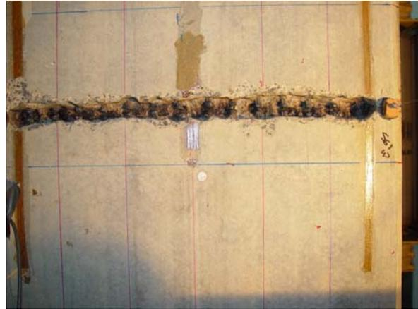
Figure 23: Modified cross section showing cut prestress strands for tests 6 & 8
