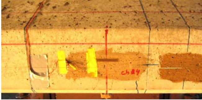
a) Flexural cracking of bottom flange
