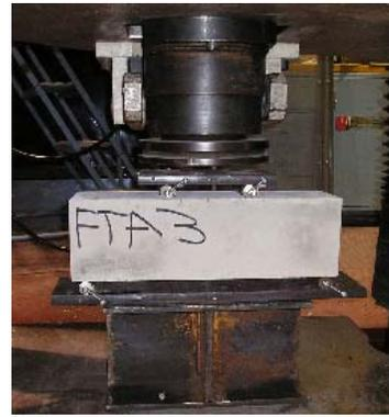
b) Modulus of rupture
