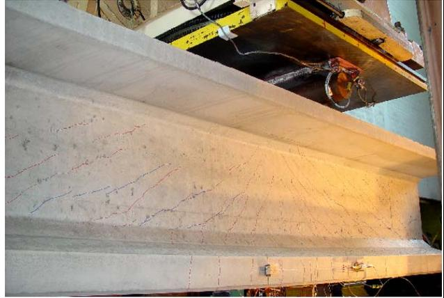
b) Flexure and shear cracking (North face)
