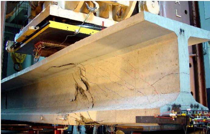
d) Shear failure (North face)
