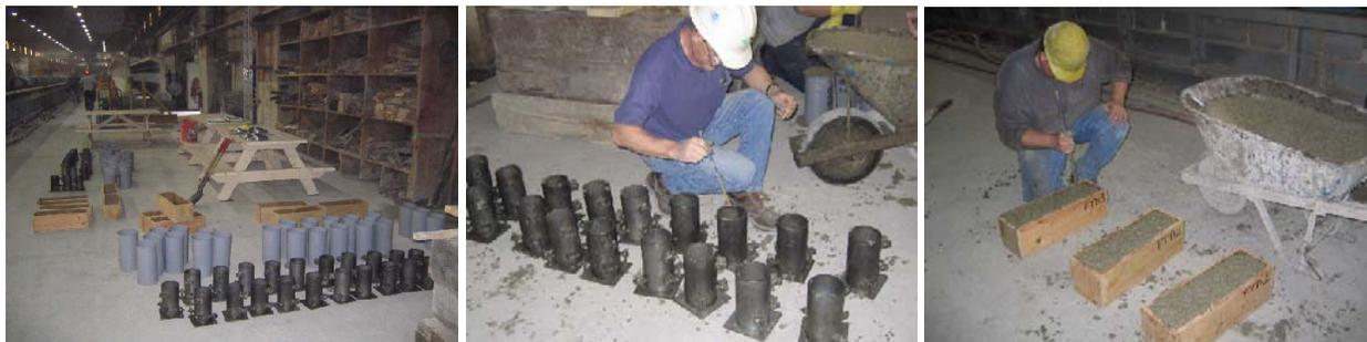
Figure 7: Cylinder and prism fabrication
