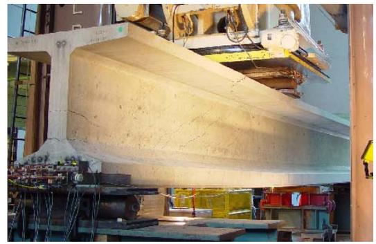
d) Local failure of top flange
