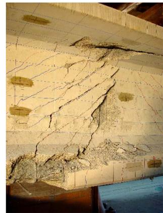
e) Shear failure (South face)
