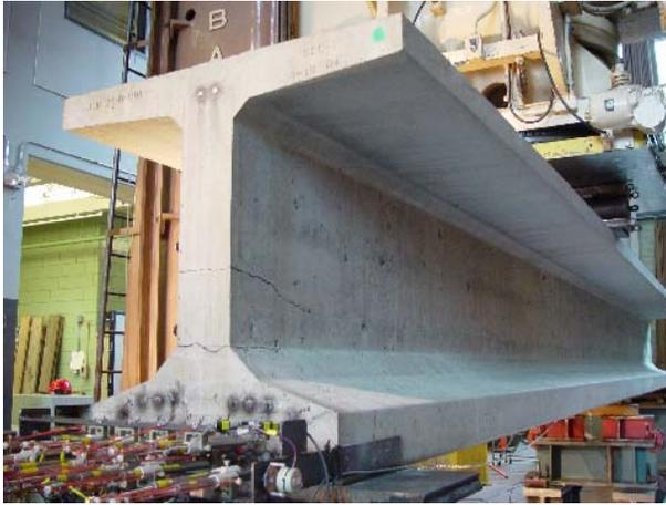
a) Initial configuration: horizontal end cracks
