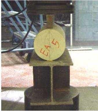
a) Splitting tension test
