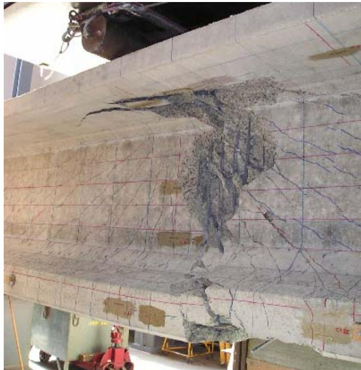
f) Abrupt shear failure of beam
