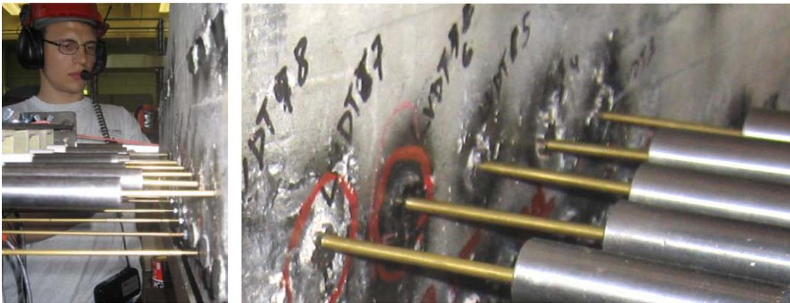
Figure 48: Slip LVDT contact
