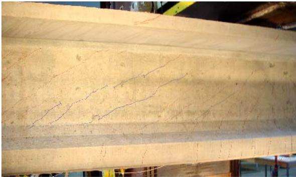
c) Flexure and shear cracking
