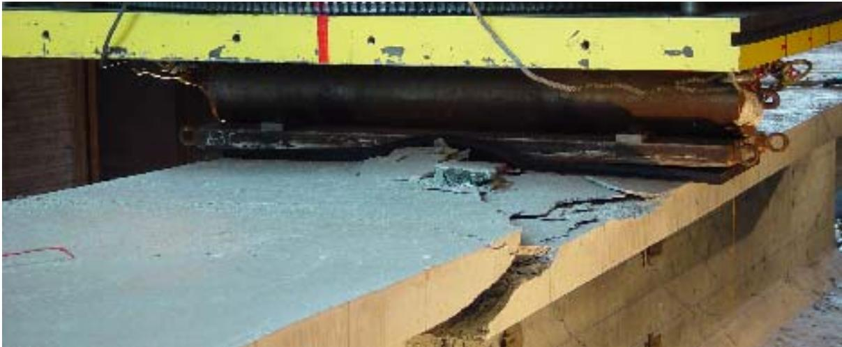
e) Local failure of flange
