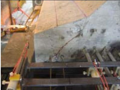
e) End splitting cracks
