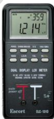
Figure 32. Example of a handheld instrument as a pragmatic solution for performing the AC impedance measurements of EIT (ESCORT ELC-131D).
