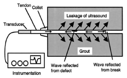
Pulse-echo test configuration for the inspection of post-tensioning steel using guided ultrasonic waves (Beard, Lowe and Cawley, 2003)
