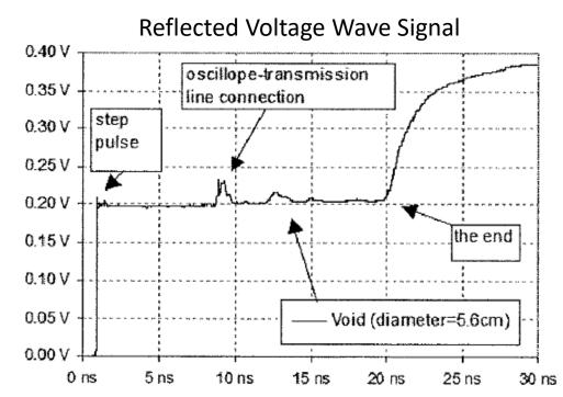
Hunsperger, R. & Chajes, M. (2006) "Void Detection in Post-Tensioning Ducts Using Time Domain Reflectometry" Highway IDEA Project 98
