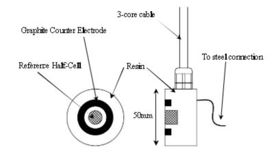
Corrosion potential and corrosion rate probe (C-Probe, Model CP101)
