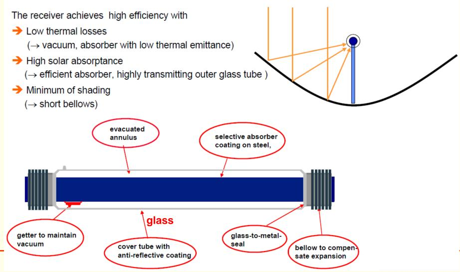
The metal receiver should be designed to minimize heat loss. Heat retention by the receiver is enhanced by covering the metal receiver with a selective (low-E) coating which will absorb virtually all the concentrated radiation, but will reradiate little energy back.
