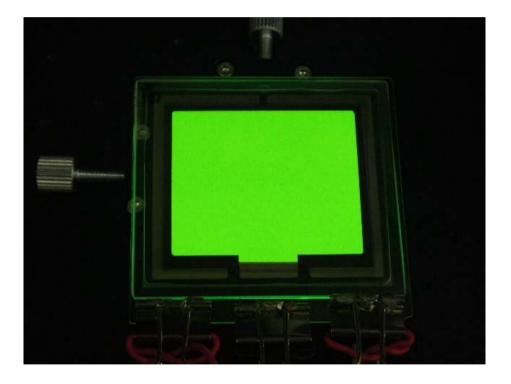
Device structure Glass /IZO,100/ND1501,40/NPD,50/Ir(ppy)3+CBP[6%],30/BAIq,10/AIq,30/LiF,0.8/AI,150
