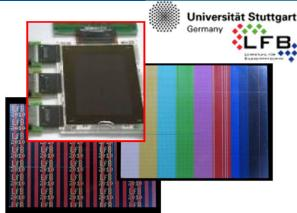
Color LCD, 4" diag., <170 $\mu$ m thick, qVGA
