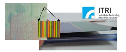
Color ChLCD, 5" diag., <210µm thick, 80ppi
