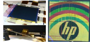
Color EKD, 3.5" diag., 3-layer stacked, <0.7mm D.A. Mourey, et al., "Amorphous Oxide Transistor Electrokinetic Reflective Display on Flexible Glass," IDW 2011.
