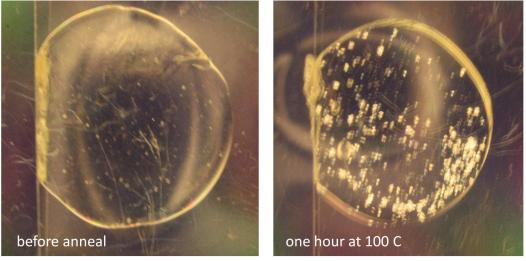
Figure 10. Photograph of crystal growth (right) in a sugar glass sample after one hour at 100°C. The sample on the left is the identical sample prior to heating. Photos taken with low cost Digital Blue computer microscope.
