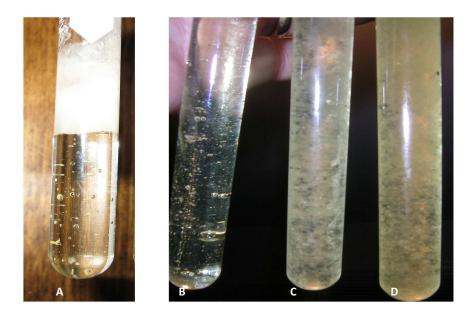
Figure 7. (A) Growth of crystals at the surface (top) of sugar glass in test tube at room temperature after several weeks of high humidity. The photo on the right shows the progression of bulk crystallization from an unheated clear candy glass (B), to one that is heated in a home oven set to  $250^{\circ}$  F ( $120^{\circ}$ C) for approximately 20 minutes (C & D).
