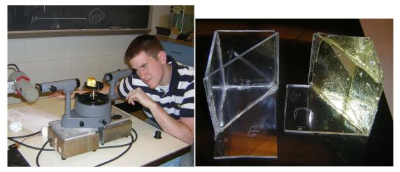
Figure 4. Left, an REU student measures the refractive index of a candy glass prism. Right, empty and candy filled prism molds made from microscope slides by the student.
