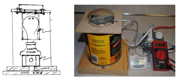
Figure 9. Sketch of the light bulb sample oven for the crystallization vs. temperature studies. (Right) Photograph of the complete apparatus with dimmer control, digital thermometer and digital volt meter (DVM) for monitoring voltage across light bulb heating element.
