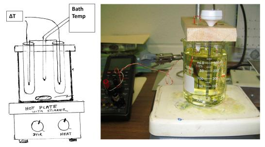
Figure 12. Sketch of the arrangement of a student-built DTA apparatus, together with the photo of a simple implementation with digital thermometer for bath temperature, and a single thermocouple meter for measuring the differential temperature.
