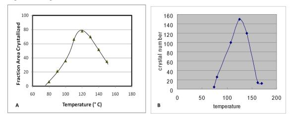
Figure 11. Examples of data measured in two different student experiments. Crystal growth rate vs. temperature in A) done by a college level REU student using Image J to extract the area from photos while B) performed by a high school student using the simple method of estimating the number of "crystal spots". Note the distinct maximum near 120° C for both approaches.
