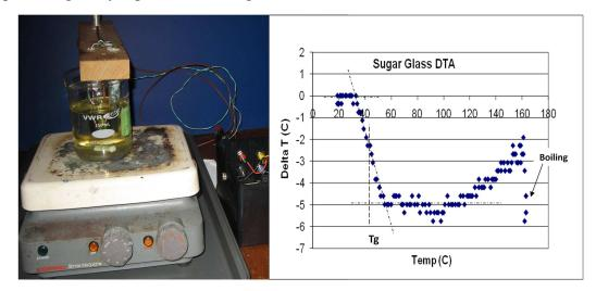
Figure 13. Photograph of the DTA apparatus with Basic Stamp microprocessor for temperature measurement and data logging. A sample DTA scan for the candy glass is shown on the right, with midpoint  $T_g$  indicated.
