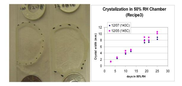
Figure 8. Photograph of crystal growth on outer edge of two samples taken on day 5 after placing in the 50% RH chamber. Note the uniform thickness of the crystal layer in both samples. On right, data show increasing width of crystal layer with time for a standard recipe glass. Two different batches are included (diamonds and squares). Note that the 145° C sample (squares) also includes a replicate.
