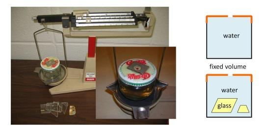
Figure 2. Low cost apparatus for the measurement of density of irregular shaped solids, using Archimedes method.
